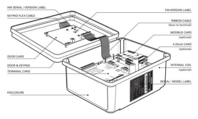
The PF2100 was designed for a product life of 10 years with some over protection margin built-in. The electronics components and parts were sourced from manufacturers with 10-year reliability criteria. Also, the availability of parts was forecasted for 10 years. Improper grounding has been the main cause of premature electronic component failures.
